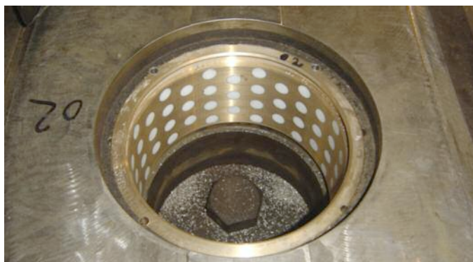
Embedded with solid PTFE, the DB spherical bearings are self-lubricating
